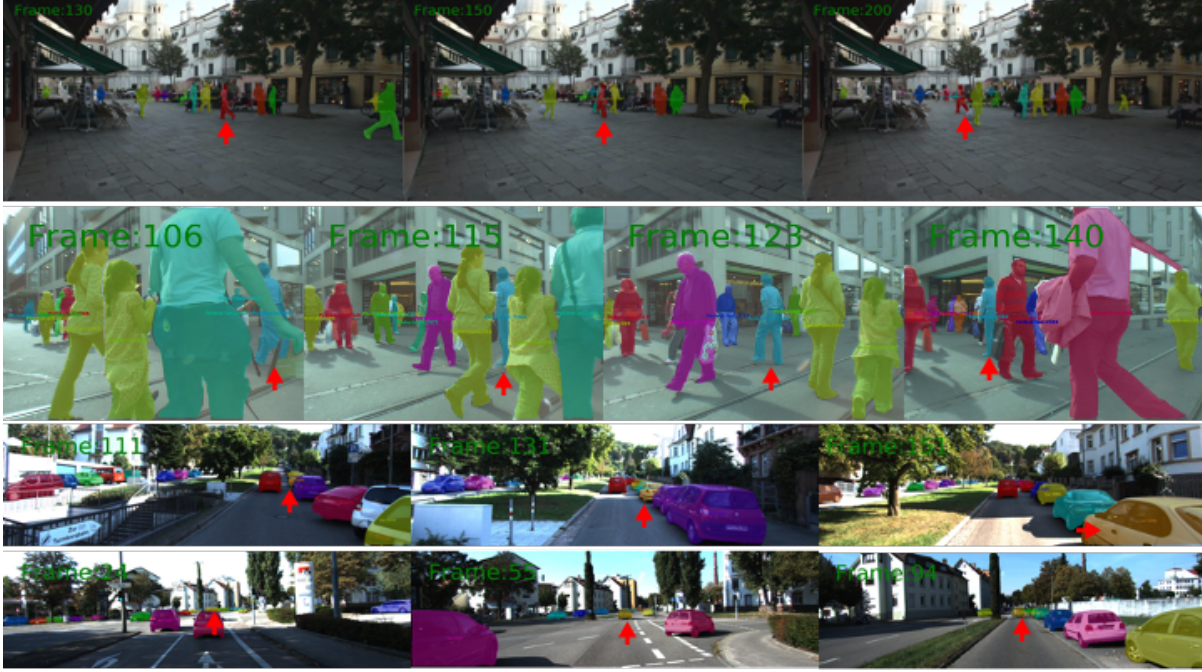
Figure 2. Qualitative results of the proposed IA-MOT. 1 st row: MOTS20-01 (static camera); 2 nd row: MOTS20-06 (stroller-mounted camera); 3 rd row: KITTI-MOTS-0011 (car-mounted camera, up-slope view); 4 th row: KITTI-MOTS-0012 (car-mounted camera, turning view). Red arrows indicate that the targets are tracked robustly even with frequent occlusion or turning.
